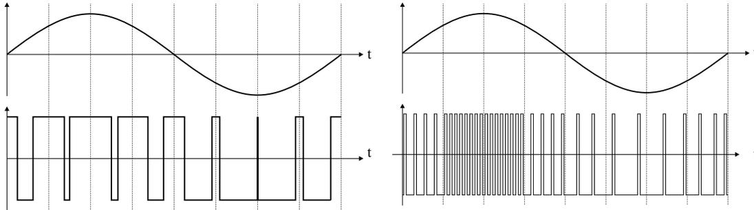
Fig. 1.10 PWM and PDM pulse modulation methods.
