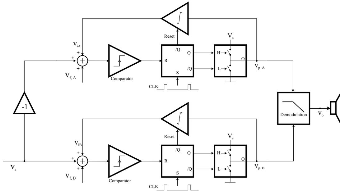
Fig. 8.3 Three-Level One Cycle Control (TOCC) effectively synthesizing NBDS PWM.
