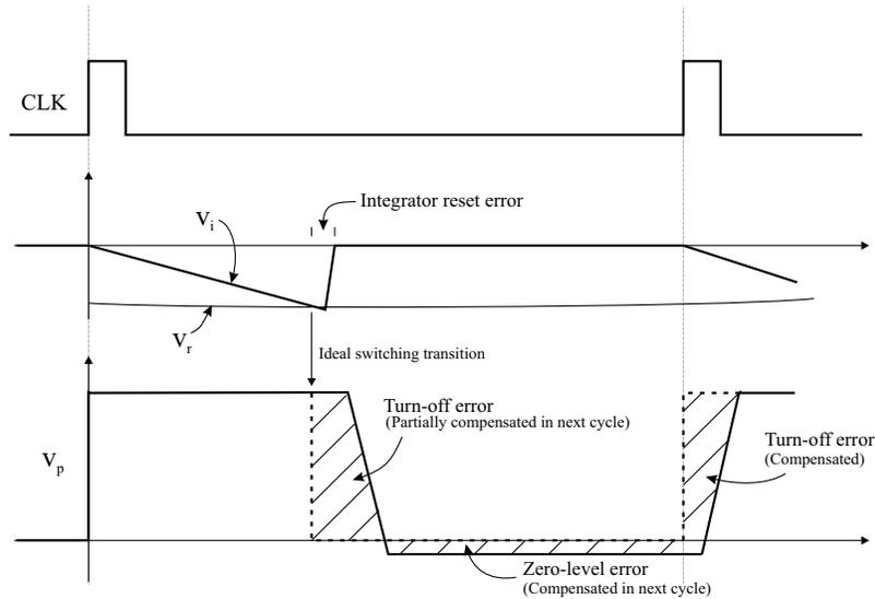
Fig. 8.2 OCC Non-linear control technique
