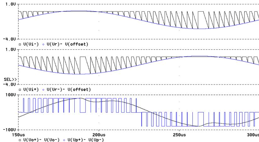
Fig. 8.10 Simulation of TOCC based system with 5% over modulation. The consequences of over-modulation are dramatic due to completely *missing* pulses as opposed to normal clipping with full (100% duty cycle) pulses.
