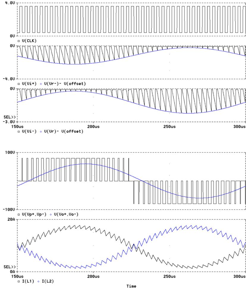
Fig. 8. 6 Functional simulation of case example with TOCC. From top to bottom: (1) Common clock, (2)-(3) control signals on both sides in terms of integrator output  $v_i$  and reference  $v_r - v_f$ , (4) Differential power stage output and demodulated output. (5) Inductor currents in the output stage illustrating the balanced drive of the load.
