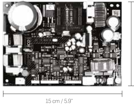
ICEpower300AS1 Amplifier and power supply 300 W @ 1 % (20 Hz - 20 kHz, 4 Ω)
